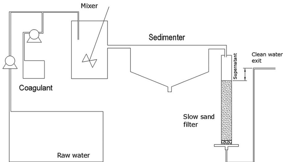
Fig. 4. Pilot plant installation.
